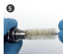
Clean the fluid nozzle internally with the correct size brush (code W2COM6126).
