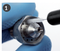
Clean small holes on the fluid nozzle with a special tiny brush (code W2COM6127).*
