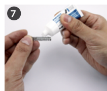
Grease the Needle spring.
