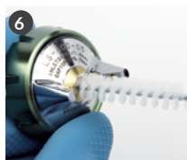
Clean the air cap center hole (code W2COM6162).
