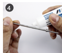
Grease the needle (code W2COM6165).
