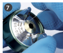
Clean the tiny holes with needle (code W2COM6164).*
