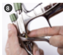
Grease the air valve bar behind the trigger.
