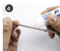
Grease the needle (code W2COM6165).
