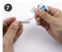
Grease the Needle spring.
