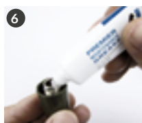
Grease the fluid adj. knob screw (code W2COM6165).
