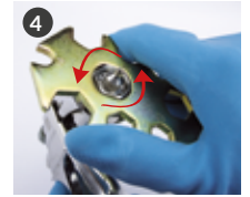
4 Unscrew the fluid nozzle with universal spanner (code 930171A0).
