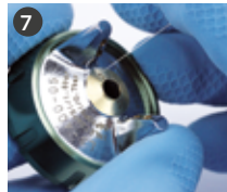
7 Clean the tiny holes with needle (code W2COM6164).*
