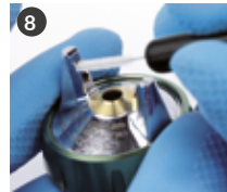
8 Clean the horn holes with special tiny brush (code W2COM6127).*
