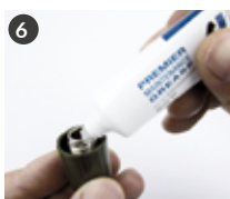
6 Grease the fluid adj. knob screw (code W2COM6165).
