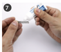
7 Grease the Needle spring.
