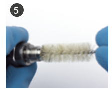
5 Clean the fluid nozzle internally with the correct size brush (code W2COM6126).
