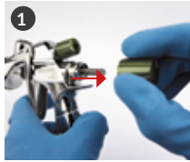
1 Take out the fluid adj. knob and needle spring.
