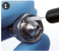
1 Clean small holes on the fluid nozzle with a special tiny brush (code W2COM6127).*
