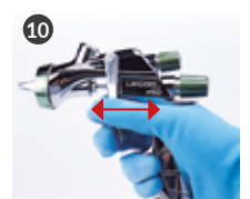
10 Check if the trigger and the needle travel smoothly.
