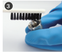
3 Clean the tip of the nozzle carefully with a brush (code W2COM6163).
