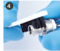
4 Clean also the thread of the nozzle carefully with a brush (code W2COM6163).
